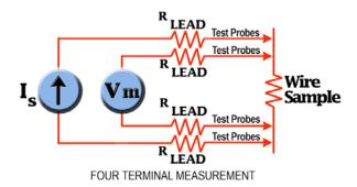
Figure 2 – The 4-terminal method is widely recognized as the preferred form of measurement.
