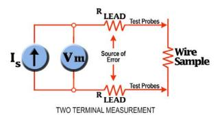
Figure 1 – The measurement method known as the 2-terminal method is subject to error introduced by  $R_{LEAD}$ .
